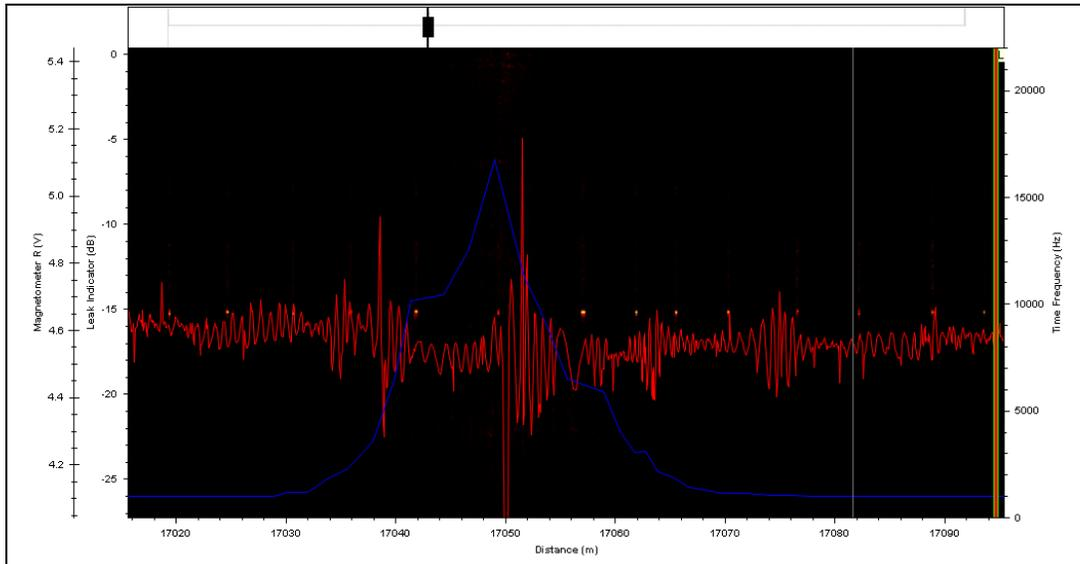
Magnetometer Output at Valve point for Simulated Leak.
