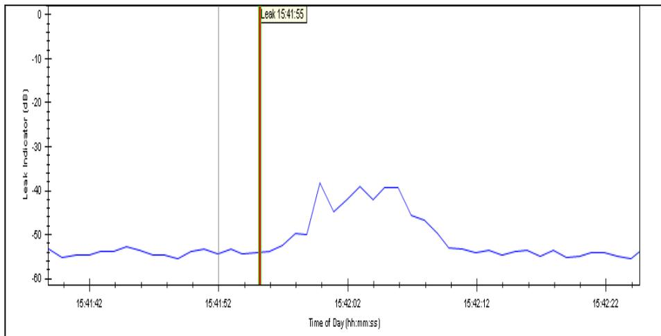
Leak Indication Power detected by the SmartBall as it passes the unknown leak.
