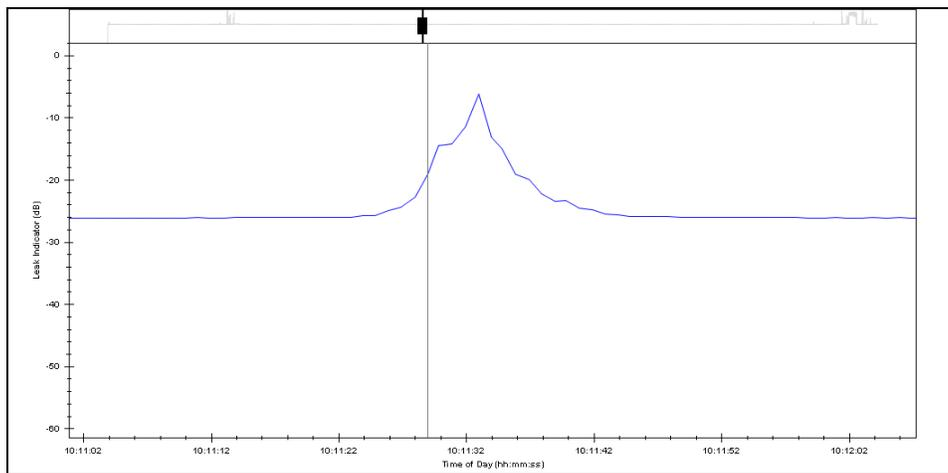
Leak Indication Power detected by the SmartBall as it passes the first simulated leak.
