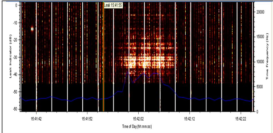
Frequency spectrum detected by the SmartBall as it passes the unknown leak.
