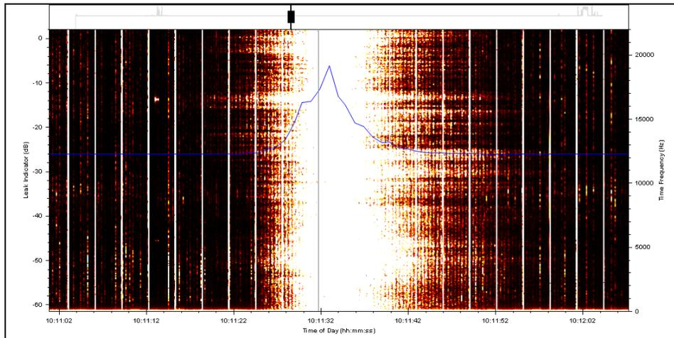
Frequency spectrum recorded by the SmartBall as it passes the first simulated leak.
