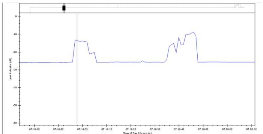
Leak Indication Power detected by the SmartBall as the second calibration leak was simulated with the ball stationary inside the insertion trap.
