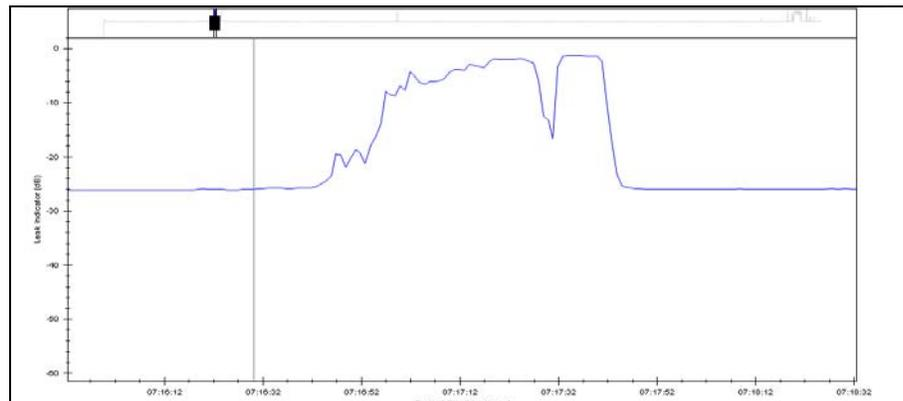
Leak Indication Power detected by the SmartBall as the first leak was simulated with the ball stationary inside the insertion trap.
