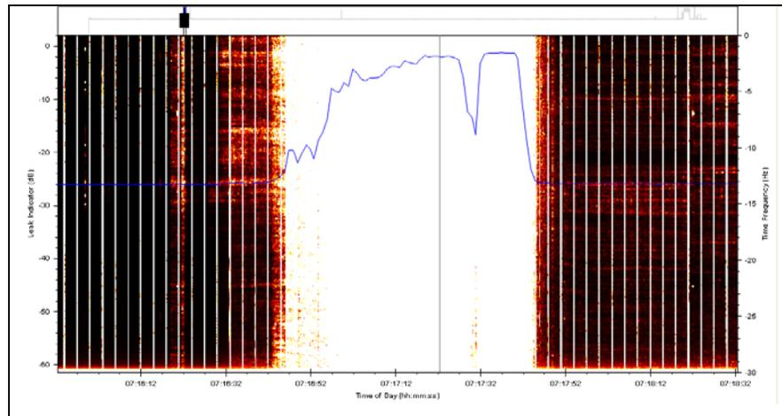
Frequency spectrum recorded by the SmartBall as the first calibration leak was simulated with the ball stationary inside the insertion trap.
