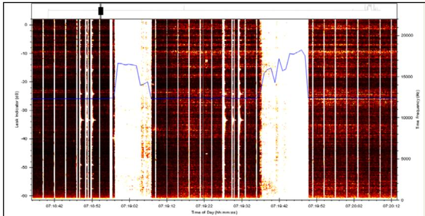
Frequency spectrum recorded by the SmartBall as the second calibration leak was simulated with the ball stationary inside the insertion trap.
