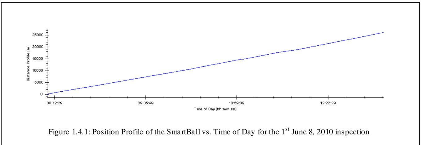
Figure 1.4.1: Position Profile of the SmartBall vs. Time of Day for the 1<sup>st</sup> June 8, 2010 inspection
