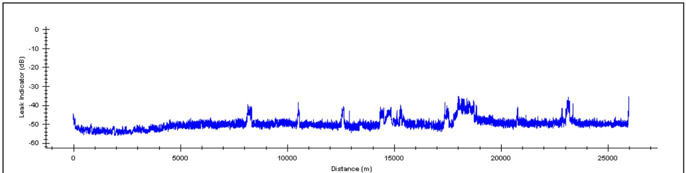
Figure 1.4.12: Acoustic Profile of the Smart Ball vs. Distance Traveled for the 1<sup>st</sup> June 8, 2010 inspection
