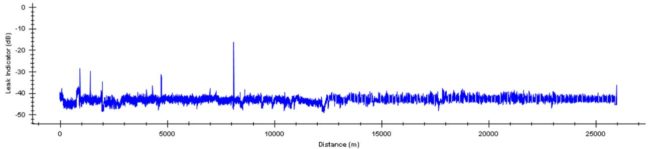
Figure 1.4.14: Acoustic Profile of the Smart Ball vs. Distance Traveled for the 3<sup>rd</sup> June 8, 2010 inspection
