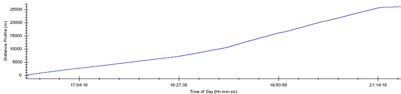
Figure 1.4.9: Position Profile of the SmartBall vs. Time of Day for the 4<sup>th</sup> June 8, 2010 inspection
