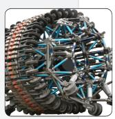
Magnetic flux leakage (MFL) is used to detect corrosion and pitting in lined metallic pipelines.
