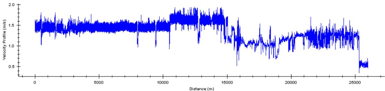
Figure 14.5: Velocity Profile of the SmartBall vs. Distance Traveled for the 2<sup>nd</sup> June 8, 2010 inspection
