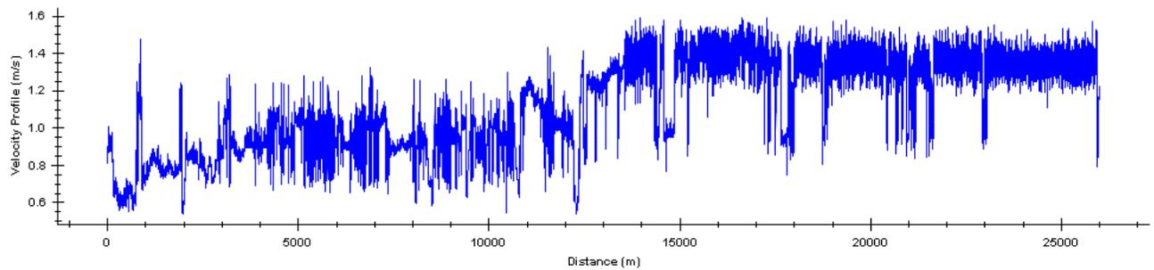
Figure 1.4.8: Velocity Profile of the SmartBall vs. Distance Traveled for the 3<sup>rd</sup> June 8, 2010 inspection
