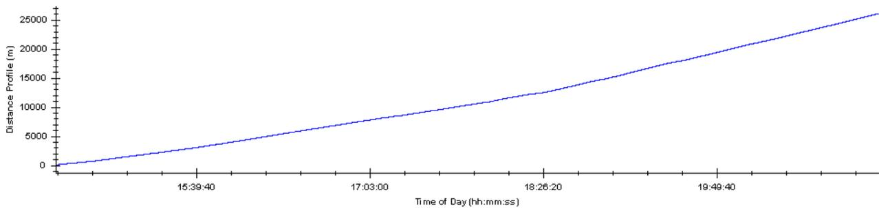
Figure 1.4.6: Position Profile of the SmartBall vs. Time of Day for the 3<sup>rd</sup> June 8, 2010 inspection
