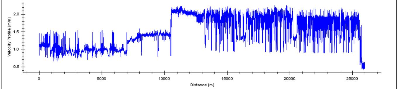
Figure 1.4.11: Velocity Profile of the SmartBall vs. Distance Traveled for the 4<sup>th</sup> June 8, 2010 inspection
