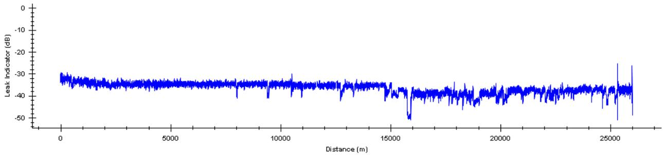
Figure 1.4.13: Acoustic Profile of the Smart Ball vs. Distance Traveled for the 2<sup>nd</sup> June 8, 2010 inspection
