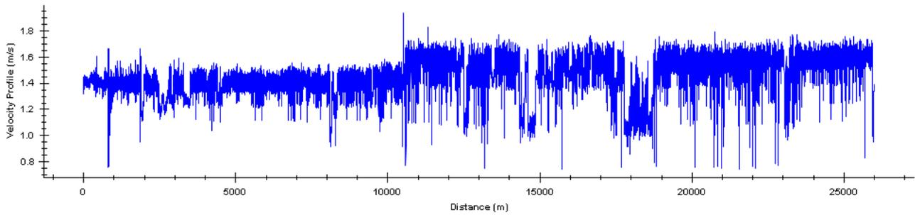
Figure 1.4.2: Velocity Profile of the SmartBall vs. Distance Traveled for the 1<sup>st</sup> June 8, 2010 inspection
