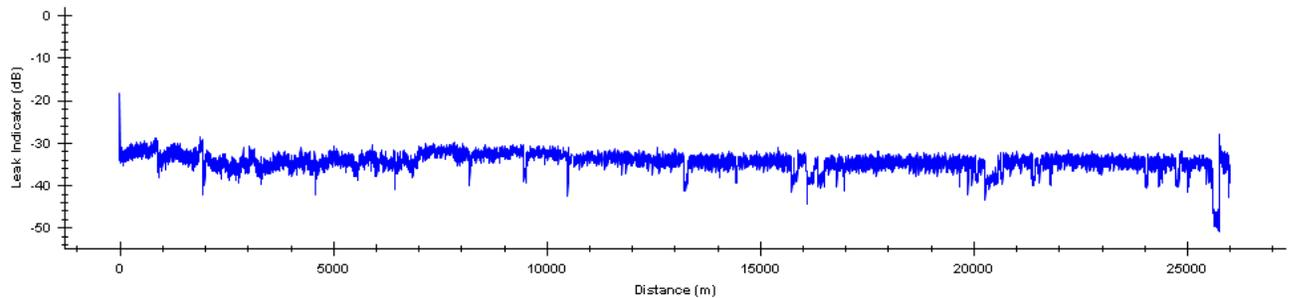
Figure 1.4.15: Acoustic Profile of the Smart Ball vs. Distance Traveled for the 4<sup>th</sup> June 8, 2010 inspection
